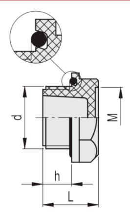
$\begin{array}{lll} d & = M \, 33x1.5 \\ D & = 44 \\ h & = 13 \\ L & = 23 \\ M & = 31 \\ s & = 38 \\ Weight (g) = 18 \end{array}$
